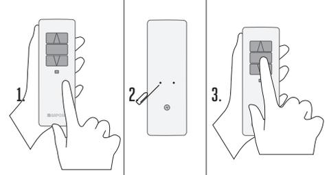
1. Press **UP** or **DOWN** the motor should go **UP** or **DOWN**, otherwise to change direction:
