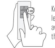
Keep the **STOP** button pressed at least for 3 seconds: the shade/awning will move till it reaches the intermediate position.
