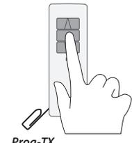
Using an programmed remote press and hold both **PROG-TX** and **STOP** buttons until the motor makes first a brief jog and, after a while, a second long jog. Memory is now empty.
