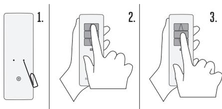
1. Push **PROG-FC** until the motor makes a brief movement in both directions
