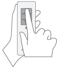
For limits set with torque sensor (mechanical stop of cassette awnings/shades), press and hold **UP** button until the bottom bar hits the cassette or shade box.
