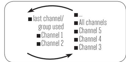
Once the desired channel selected, you can proceed to activate the corresponding motor by using **UP**, **STOP** and **DOWN** buttons. Moreover, you can also memorize up to 8 combinations of groups of channels.
