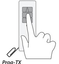
2. Within 8 seconds, using any Sun Control remote, press and hold both **PROG-TX** and **STOP** buttons until the motor makes a long jog. Memory is now empty.
