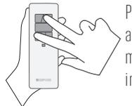
Press simultaneously the **UP** and **DOWN** buttons until the motor makes a brief movement in both directions.
