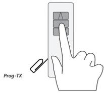
Push simultaneously **PROG-TX** and **STOP** of the remote until the motor makes a brief movement in both directions.
