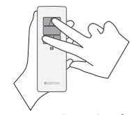
Stop the shade/awning in the desired intermediate position, then press simultaneously the **UP** and **DOWN** buttons until the motor makes a brief movement in both directions. The intermediate position has been setup.
